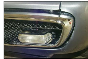
Figure 21. From bumper light locations. Early versions are on the left. For 1968 through about 1970, the Carello lights were moved to the top of the grille opening. Later cars had a cheaper looking plastic light mounted on the bottom of the grille.
