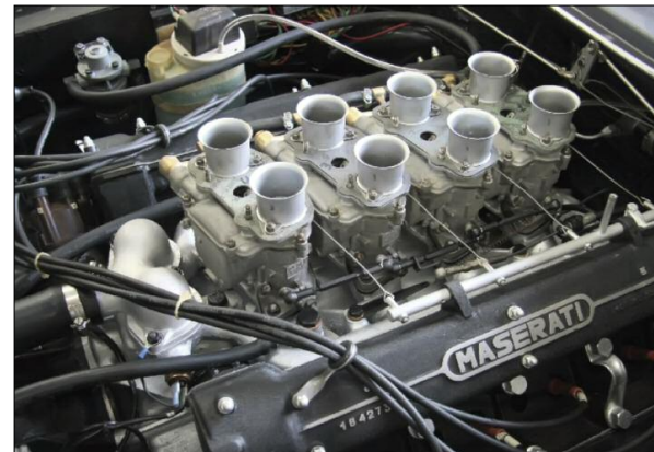
Figure 22. Early V8 with the DCNL carburetors. The Maseratis seem to have as much beauty under the hood as outside. Courtesy of Ivan Ruiz.
