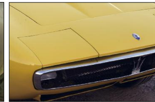
Figure 21. From bumper light locations. Early versions are on the left. For 1968 through about 1970, the Carello lights were moved to the top of the grille opening. Later cars had a cheaper looking plastic light mounted on the bottom of the grille.
