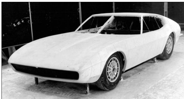
Figure 5. An early Ghibli studio form that appears to be made from clay used to evaluate the design concept and plan for production (Courtesy of Maserati North America).
