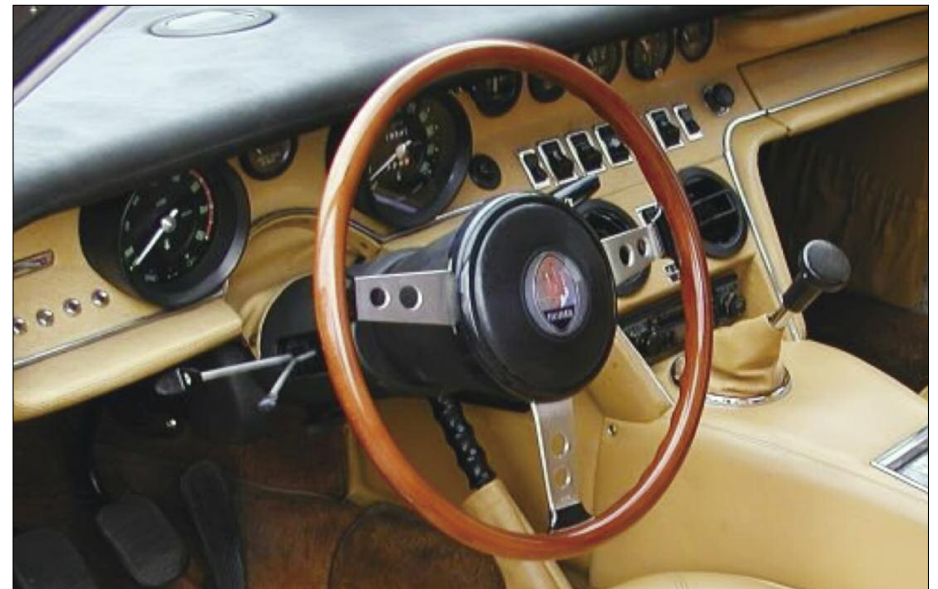
Figure 17. Later dash board configuration (actually from a SS model) with rocker switches and padded steering wheel. Courtesy of Ivan Ruiz.
