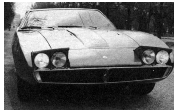
Figure 8. Front shot of the Ghibli with the lights lifted. The early bodies, like the prototype, lacked additional air inlets for the radiator. (Source: Road and Track 1967)
