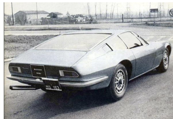
Figure 7. This side shot of the Ghibli prototype shows the lack of exterior production door handles and the early drop down trunk. The exhaust, bumpers and side trim are much as they were on early production models. (Source: Road and Track 1966)
