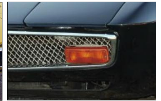
Figure 21. From bumper light locations. Early versions are on the left. For 1968 through about 1970, the Carello lights were moved to the top of the grille opening. Later cars had a cheaper looking plastic light mounted on the bottom of the grille.
